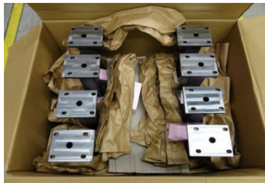
Figure 4: Inadequate packaging (oversized box, items are not secured)
