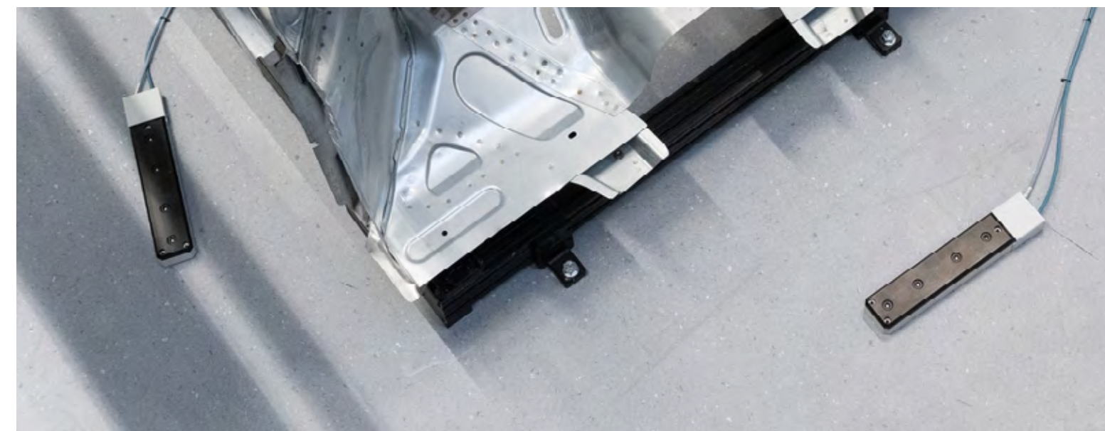
Stability modules on the ground are fixed reference for the tracking system even with temperature fluctuations in the production environment.
