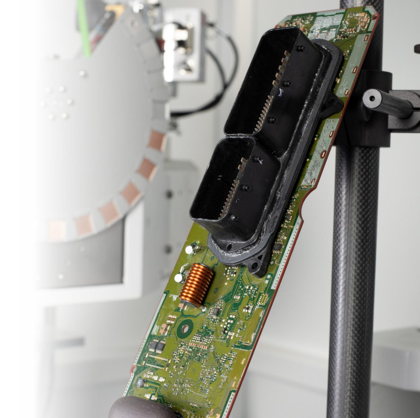
Power Electronics Connection Non-destructive Inspection by CT
