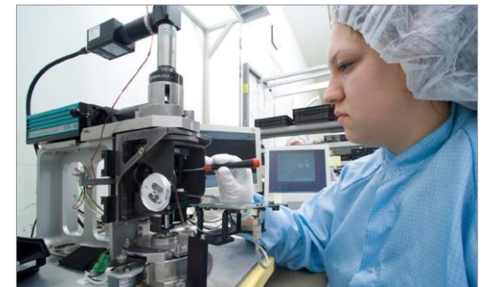
The zoom body adjustment device calculates the zoom control curve from around 7,000 reference points.
