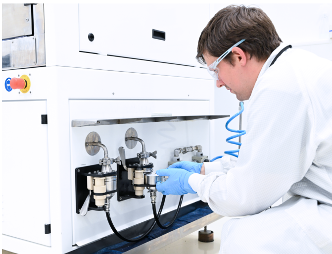
The filters are collected at the outlet and analyzed microscopically.
