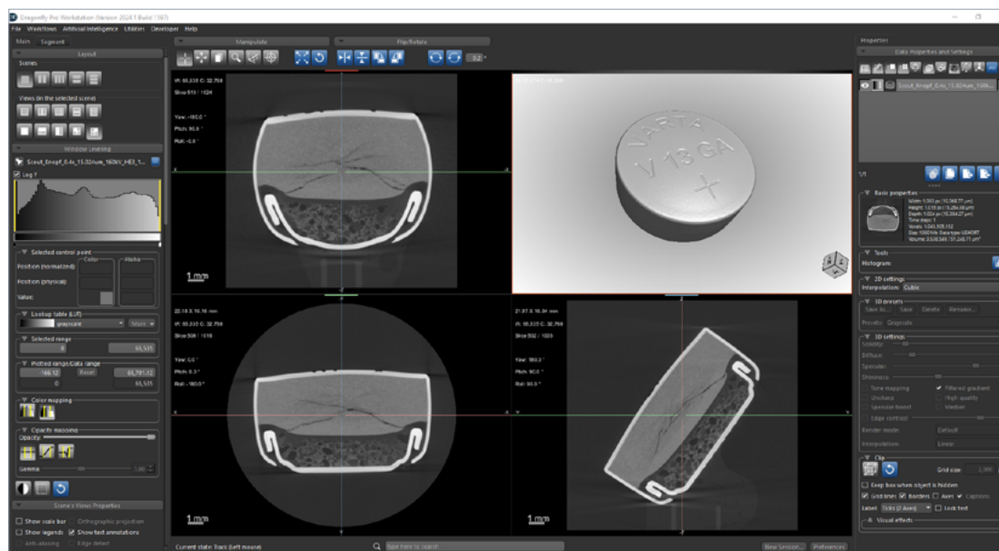
Tailor tools that are optimal to your workflow: choose plug-ins that allow you to control registration, map differences, and customize appearance. Commercial button cell battery, imaged on a ZEISS Versa XRM.
