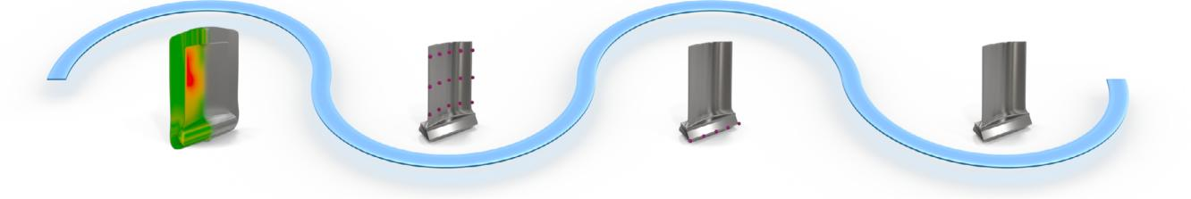
The final machining ensures the part is fit for it's intended final use. The airfoil edges with the small radii for performance, the root form for fit to the compressor disc and airfoil tip to ensure no leakage of compressed gas.
