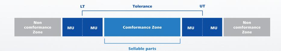
ZEISS Original Accessories enable you to reliably deliver high quality products by minimizing the measurement uncertainty (MU) for each individual measuring point.
