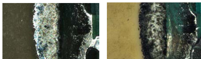
PCB component: without Polarizer Unit (left); with Polarizer (right).
