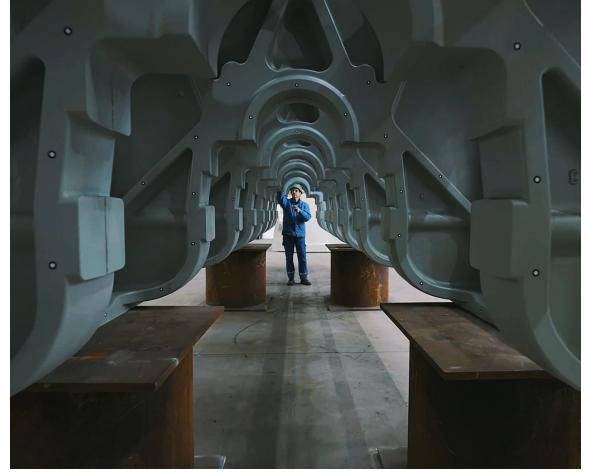
The German Siempelkamp Gießerei has installed the world's largest non-contact robot measuring cell together with ZEISS, to ensure precise quality of their very large castings.
