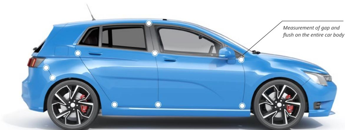
E.g. gap and flush on the painted car body with nine measuring points (gap specifications: in the range of 3,4 mm  $\pm$  0,5 mm to 4,4 mm  $\pm$  0,5 mm).
