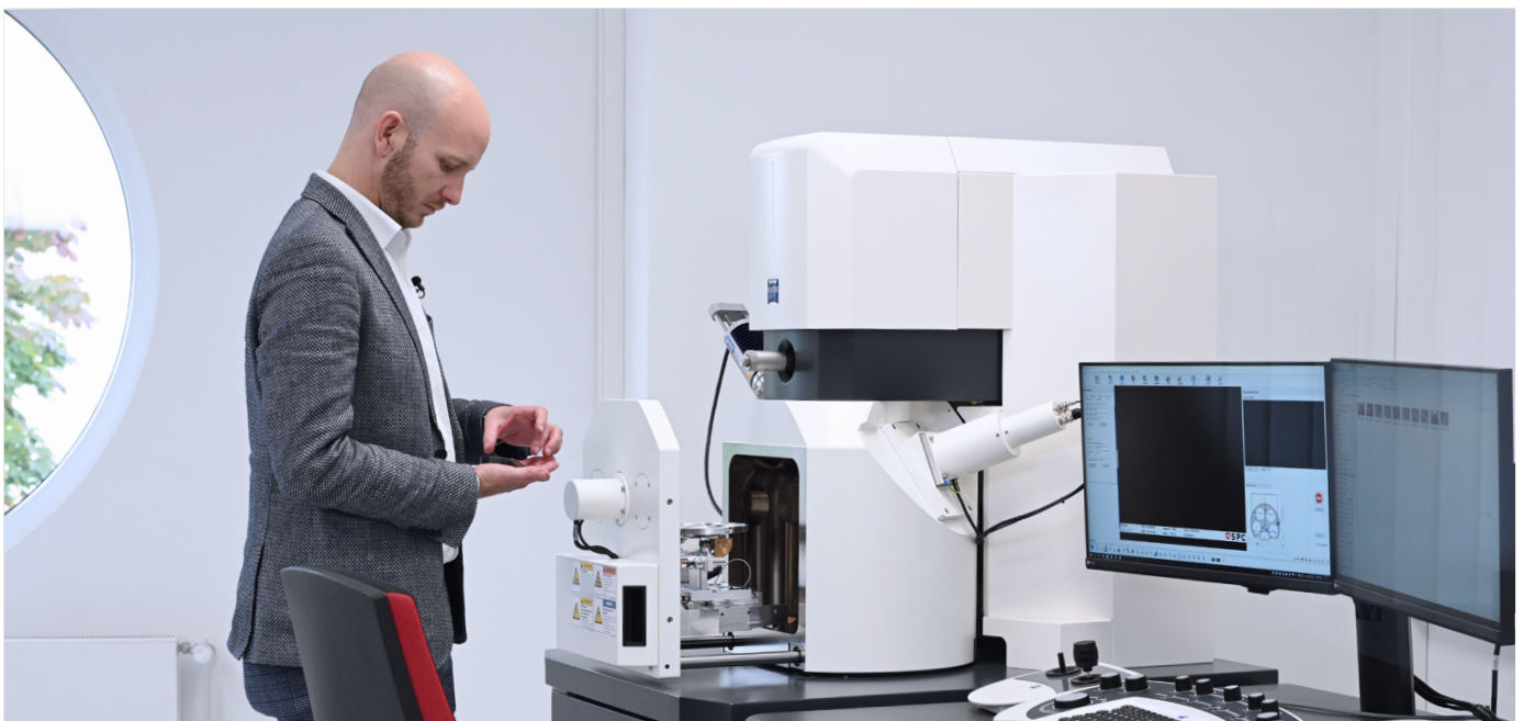
The final step was to identify which materials the contamination consisted of. To do this the employee examined a metallographic section of the pinion shaft using the ZEISS EVO scanning electron microscope.
