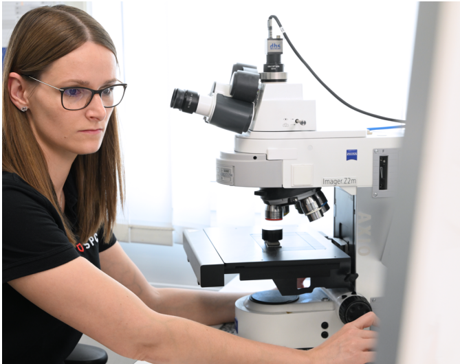
The sample is examined using the ZEISS Axio Imager, a high-resolution wide-field microscope for automated materials research.
