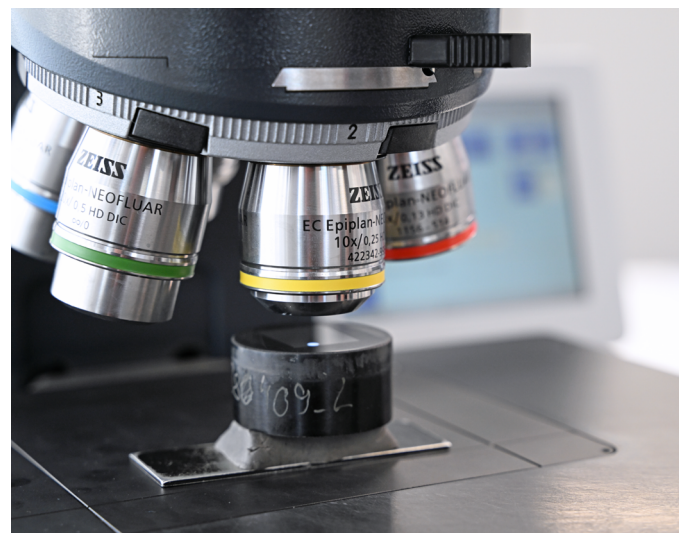
In order to analyze the microstructure inside even more precisely, a metallographic section is produced.
