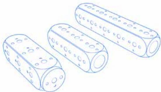
Multiple mounts are milled for stylus holders that are available in different designs. Almost any shape can be realized, from beams to complex angle elements. Due to the high complexity of the requirements, the standard portfolio in the M5 range is limited to the most common shapes. Greater flexibility can be achieved by using M5 pro elements.
