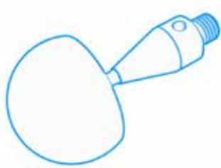
Hemisphere styli are suitable for measuring undercuts as well as for those applications that require a large diameter of the stylus tip with low weight. To enhance this effect, n is a distinction made between hemispherical and hollow hemispherical styli. Hollow hemispheres are produced using a complex manufacturing process in order to achieve maximum weight savings. For VAST XXT probes, hemisphere styli are not suitable for weight reasons. Only hollow hemisphere styli are used here.
