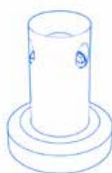
Swivel elements, such as articulated elements, are used to create angled combinations. The angle is adjusted to the main axis of the articulated element. Rotating elements are available as a complete rotating unit or as basic elements with a cone holder (CR); connecting elements with a cone adapter (CA) can be adapted.
