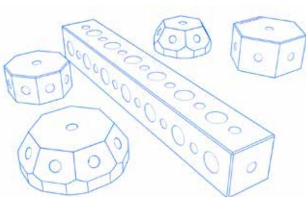
Multiple mounts are milled for stylus holders that are available in different designs. Almost any shape can be realized, from beams to complex angle elements. Due to the high complexity of the requirements, the standard portfolio in the M5 range is limited to the most common shapes. Greater flexibility can be achieved by using M5 pro elements.
