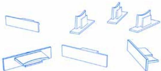
If different stylus systems are used in a measuring program, they must also be noted accordingly in the programming. For this purpose, each stylus system has its own designation, which can be selected by the user. In order to distinguish them from each other, the stylus systems themselves should also be appropriately labeled. To do this, identification labels such as these are simply attached to the adapter plate
