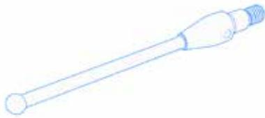
Clamping styli have an extended adapter compared to conventional styli. This means that it consists of the actual adapter and a fitting cylinder between the adapter and the thread. This allows the M3 XXT star elements to be clamped directly via the stylus in the same way as with a clamping screw. The other dimensions of the stylus correspond to those of the comparable standard stylus
