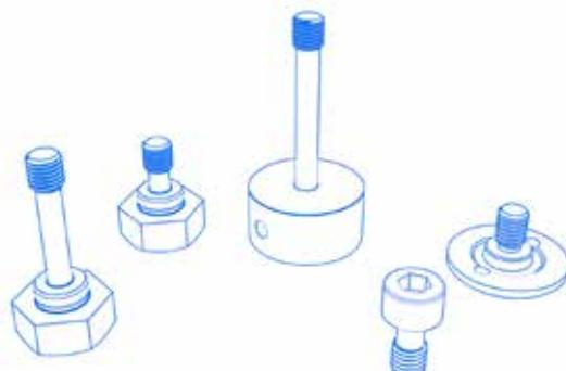
Screws for fixing and adjusting a wide variety of connecting elements and disk styli. Undercut screws can be screwed through cubes into an extension. This makes it possible to adjust the angle of the subsequent component. The required length of the screw depends on the thickness of the inserted cube.
