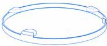
These protective rings are used to protect the adapter plates from damage during setting-up and measuring operations or during storage. The collision protection rings are made of plastic and are simply slipped over the aluminum body of the adapter plate. This protects the sensitive edges from shocks and extends the life of plates.
