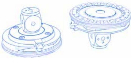
These adapter plates are comparable to the standard XTR adapter plates. Instead of an M5 thread, however, they also have M5 pro index holes, so that all elements from the M5 pro system can be connected. They can also be used for all standard M5 elements. They consist of the XTR base body and direct adaptation with M5 threads and index holes in the Z direction or a 22 mm cube with M5 threads and index holes for receiving M5 and M5 pro elements. Usable for measuring head VAST XTR Gold
