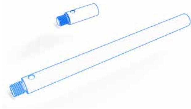
Standard M3 extensions have a smaller outer diameter of 4 mm compared to the 5 mm diameter used with the ZEISS M3 XXT system. The resulting loss of rigidity is compensated for by the use of a stable titanium rod. The weight of these extensions is lower than comparable extensions made of stainless steel, but still significantly higher than ZEISS M3 XXT systems
