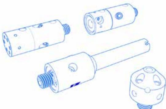
Clamp holders are used when styli without threads are used. Even if the stylus breaks, the holder can be reused. Clamp styli are available in different designs. They are usually used as holders for star styli. L-styli and adjustable angle styli can also be found in the portfolio.
