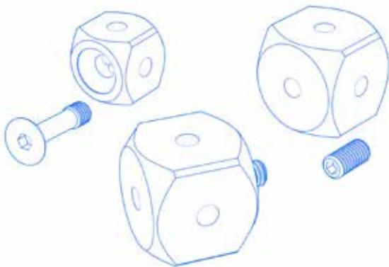
Cubes are the most common connecting element in a stylus system. ZEISS has a wide range of different designs for all applications in its portfolio. From the simple L-cube with one connection option to multiple cubes, which are used for gear measurement without a rotary table, among other things. In contrast to the rotationally adjustable elements, standard cubes are not equipped with a cone adapter and are fixed either with the integrated screw or with an additional screw.
