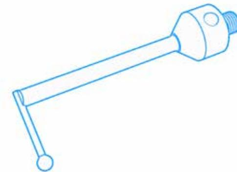
With L styli, by default the stylus tip is at a 90° angle to the stylus shaft. Due to their L shape, the styli are particularly well-suited for measuring undercuts in bores. Furthermore, an L stylus can also be used to measure difficult-to-reach points (e.g. on the underside of the workpiece). In addition to the 90° angle, other angular positions are also possible
