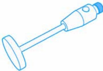
Disc styli are used, among other things, to measure rotationally symmetrical workpieces with undercuts or recesses and bores. However, a strong filtering of the surface roughness usually occurs. With the design of the spherical disk stylus, a higher accuracy is achieved compared to disk styli.
