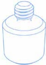
Measuring sensors are not only limited in terms of attached weight, but also in terms of the moment in force. If a probe system protrudes too far in one direction, then it is necessary to adapt a counterweight on the opposite side to reduce the tipping moment. However, you must still be careful not to exceed the permissible total weight of the probe system. For VAST/VAST gold probe heads, a tipping moment maximum of 0.1 - 0.3 Nm is permitted.
