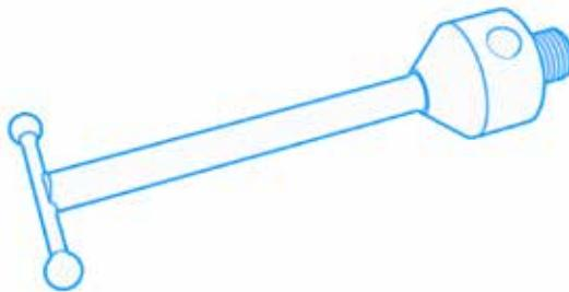
T-styli consist of two opposing measuring probe spheres mounted at 90° to the shaft. These styli are particularly suitable for measuring opposing holes and undercuts, such as grooves. In addition, T-styli can also be used for measuring points that are difficult to access (e.g. on the underside of the workpiece).
