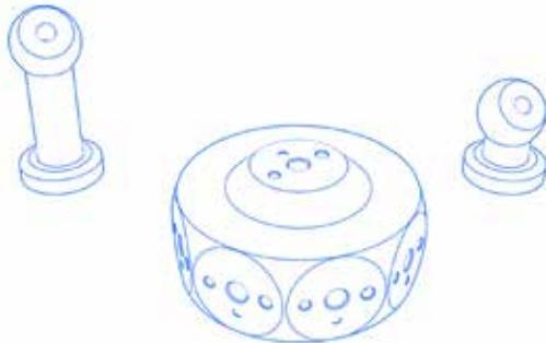
Specially manufactured angle pieces can be milled to any angle between 0 and 90 degrees. The advantage of this is that the angle cannot be changed, even in the event of a collision. These angle pieces are CNC milled and therefore more precise than flexible elements set by hand. Of course, this advantage also comes with a limitation in flexibility.
