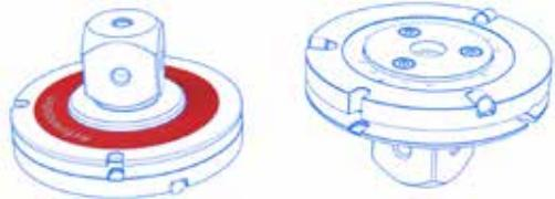
Reference adapter plates are used for the qualification of the machine and to define the reference sphere position. The reference adapter plates are marked with a red ring and should not be used for standard measurements. Suitable for probe heads VAST XT Gold, VAST Gold, VAST C-G1 and VAST XTR Gold (no rotation function).
