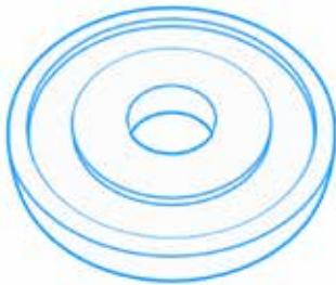
Discs are used, among other things, to measure rotationally symmetrical workpieces with undercuts or recesses and bores. However, a strong filtering of the surface roughness usually occurs. With the design of the spherical disc stylus, a higher accuracy is achieved compared to disc styli. Discs are screwed directly to extensions or special shafts using clamping disks. Normally, fastening material is not included in the delivery package
