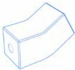
Specially manufactured angle pieces can be milled to any angle between 0 and 90 degrees. The advantage of this is that the angle cannot be changed, even in the event of a collision. These angle pieces are CNC milled and therefore more precise than flexible elements set by hand. Of course, this advantage also comes with a limitation in flexibility.
