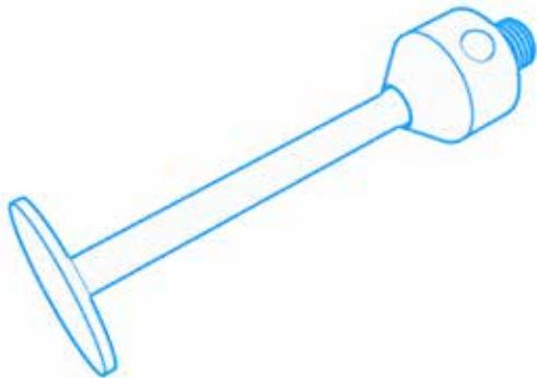
Disc styli are used, among other things, to measure rotationally symmetrical workpieces with undercuts or recesses and cylinders. However, a strong filtering of the surface roughness usually occurs. With the design of the spherical disk stylus, a higher accuracy is achieved compared to disk styli.
