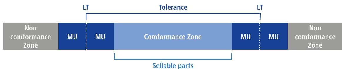
ZEISS Original Accessories enable you to reliably deliver high quality products by minimizing the measurement uncertainty (MU) for each individual measuring point.
