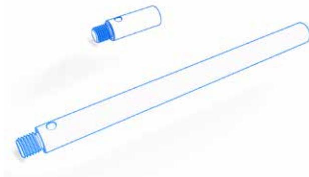
Standard M3 extensions have a smaller outer diameter of 4 mm compared to the 5 mm diameter used with the ZEISS M3 XXT system. The resulting loss of rigidity is compensated for by the use of a stable stainless steel rod. However the weight of the extensions is significantly higher compared to the carbon fiber used in the ZEISS M3 XXT system
