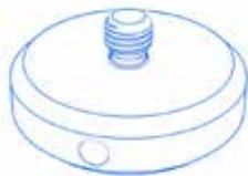
Measuring sensors are not only limited in terms of attached weight, but also in terms of the moment in force. If a probe system protrudes too far in one direction, then it is necessary to adapt a counterweight on the opposite side to reduce the tipping moment. However, you must still be careful not to exceed the permissible total weight of the probe system. For VAST/VAST gold probe heads, a tipping moment maximum of 0.1 - 0.3 Nm is permitted.
