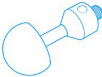
Hemisphere styli are suitable for measuring undercuts as well as for those applications that require a large diameter of the stylus tip with low weight. To enhance this effect, there is a distinction made between hemispherical and hollow hemispherical styli. Hollow hemispheres are produced using a complex manufacturing process in order to achieve maximum weight savings.
