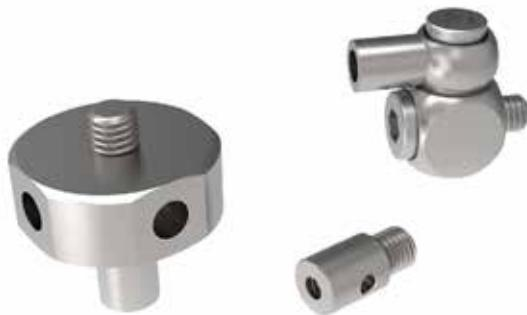
M3 REN connecting elements are used to create multiple or angled stylus combinations and star stylus with an M3 thread. The M3 REN system is based on 4 mm diameter base bodies and can only be combined with the M3 XXT system in exceptional cases using special adapters.
