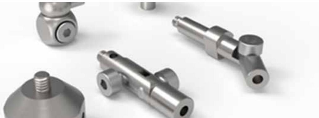
M2 connecting elements are used for the construction of multiple or angled styli combinations and star styli with M2 threads. The M2 system is based on a 3 mm diameter base body and is mainly used with M2 sensors. Use on other systems can be made possible using special adapters.
