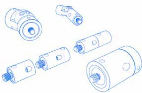
Swivel elements, such as articulated elements, are used to create angled combinations. The angle is adjusted to the main axis of the articulated element. Rotating elements are available as a complete rotating unit or as basic elements with a cone holder (CR); connecting elements with a cone adapter (CA) can be adapted.
