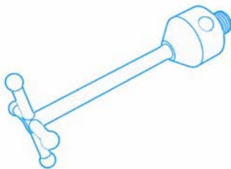
Star styli consist of spherical styli combined in a star shape and enable measurements in different coordinate directions. Whereas probing with spherical styli from the side surfaces is only possible to a limited extent, with the star stylus you can select the stylus for probing that is orthogonal to the probed surface.
