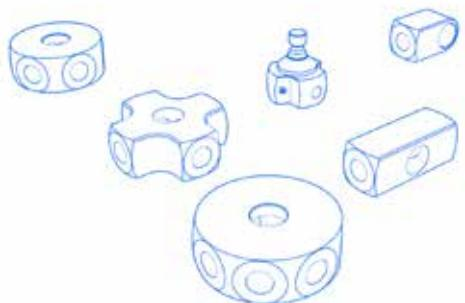
Cubes are the most common connecting element in a stylus system. ZEISS has a wide range of different designs for all applications in its portfolio. From the simple L-cube with one connection option to multiple cubes, which are used for gear measurement without a rotary table, among other things. In contrast to the rotationally adjustable elements, standard cubes are not equipped with a cone adapter and are fixed either with the integrated screw or with an additional screw.
