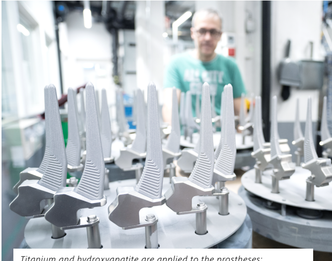
Titanium and hydroxyapatite are applied to the prostheses; the coating process took several hours.
