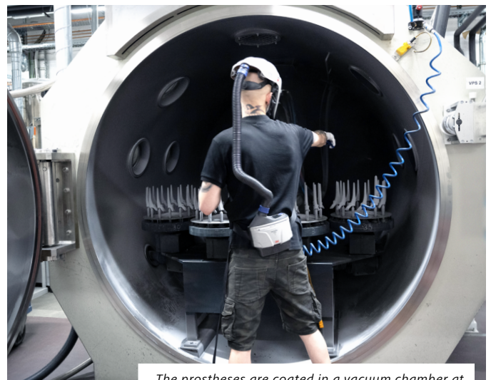
The prostheses are coated in a vacuum chamber at up to 20,000 degrees Celsius.
