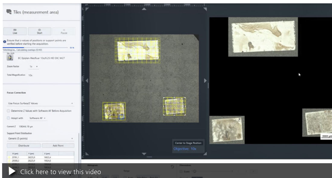
Guided Acquisition - Automatically define regions for the detail scan from an overview image
