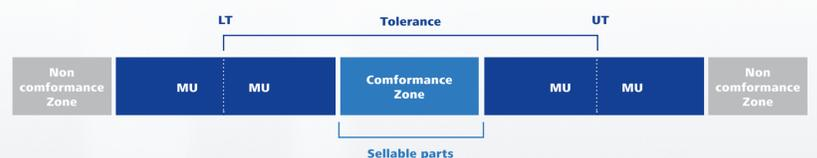
ZEISS Original Accessories enable you to reliably deliver high quality products by minimizing the measurement uncertainty (MU) for each individual measuring point.
