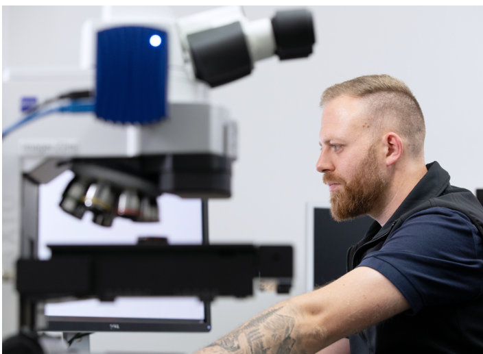
Measuring step 01: With incoming goods, a microscopic material analysis is carried out with ZEISS Axio Imager.
