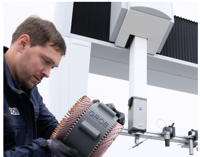
Measuring step 04: Tactile quality control on the ZEISS PRISMO verity.
