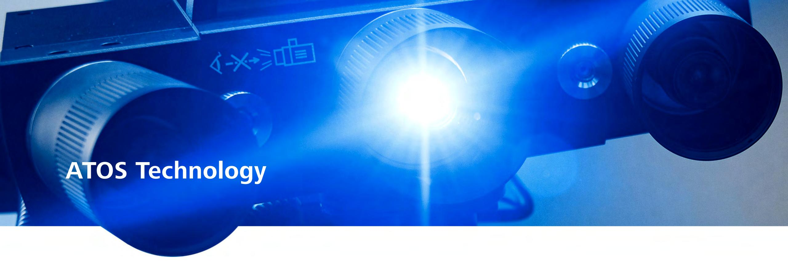
ATOS sensors are fully tailored to the metrological requirements of industrial users. Precise optoelectronics deliver absolutely accurate and traceable measurement results. Using structured blue light, the fringe projection systems enable non-contact measurements.
