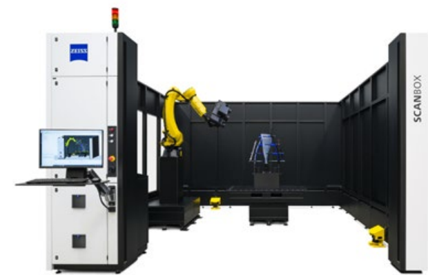
ZEISS ScanBox High throughput measurement of diverse product ranges (ribs, spars, fuselage sections)
