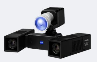
ARAMIS sensors enable the dynamic acquisition of 3D coordinates, 3D displacements and 3D surface strain. Based on triangulation, the measuring systems scan precise 3D coordinates for full-field and point-based measurements.
