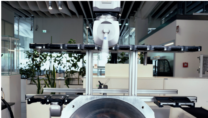
The articulating stylus replaces several configurations with fixed styli, as its stylus can swivel in one plane, motor-driven and software-controlled.
