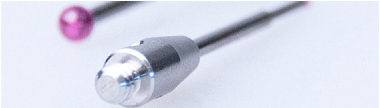
Styli with M2 thread are especially suitable for switching probes. With the appropriate connecting element they can also be connected to other thread systems. In the M2 range, styli using ruby or silicon nitride spheres are available. The shaft is made of tungsten carbide as standard. Cylindrical styli, which are made entirely of tungsten carbide, and disk styli made of ceramic, are also available.
