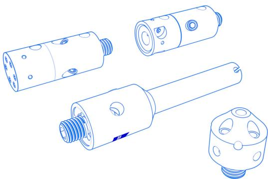
Clamp holders are used when styli without threads comes into action. Even if the stylus breaks off, the holder can be reused. Clamping styli are available in different versions. They are usually used as holders for star styli. However, L styli and adjustable angle styli can also be found in the portfolio.
