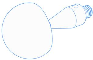
Hemisphere styli are suitable for measuring undercuts as well as for those applications that require a large diameter of the stylus tip with low weight. To enhance this effect, n is a distinction made between hemispherical and hollow hemispherical styli. Hollow hemispheres are produced using a complex manufacturing process in order to achieve maximum weight savings. For VAST XXT probes, hemisphere styli are not suitable for weight reasons. Only hollow hemisphere styli are used here.
