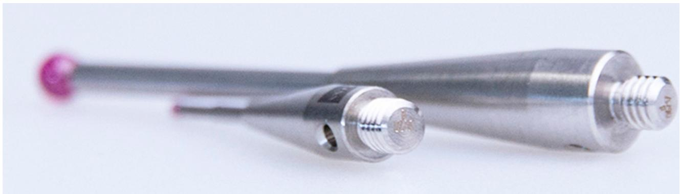
Styli with M3 thread suitable for ZEISS RST, Renishaw SP and Hexagon HP-S sensors. M3 styli can also be connected to other thread systems using the appropriate adaptors and connecting elements. Styli spheres are made of ruby or silicon nitride. In addition to the standard spherical styli, cylindrical styli made of tungsten carbide and ruby are also available. The standard straight shaft is made of tungsten carbide, but a stepped shaft is also available to provide additional stiffness.
