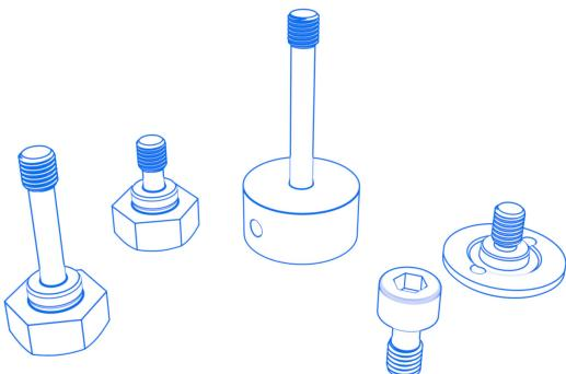
Screws for fastening and adjusting various connecting elements and stylus discs. Undercut screws can be screwed into an extension through the cube. This enables angular adjustment of the following components. The required length of the screw depends on the thickness of the inserted cube.
