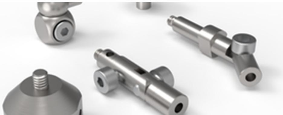
M2 connecting elements are used for the construction of multiple or angled styli combinations and star styli with M2 threads. The M2 system is based on a 3 mm diameter base body and is mainly used in conjunction with RENISHAW probes. Use on other systems can be made possible using special adapters.
