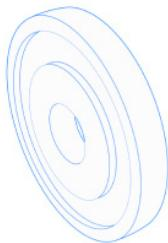
Discs are used, among other things, to measure rotationally symmetrical workpieces with undercuts or recesses and bores. However, a strong filtering of the surface roughness usually occurs. With the design of the spherical disc stylus, a higher accuracy is achieved compared to disc styli. Discs are screwed directly to extensions or special shafts using clamping disks. Normally, fastening material is not included in the delivery package
