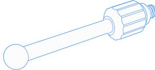
These innovative styli with plastic coated thread are a cost-saving alternative to standard styli. Their carbon fibre shaft is tipped with a ruby sphere and has been especially designed for the use with the VAST XXT probe. Beneath the cost factor there is the benefit, that these styli can be mounted without any tools. Compared to conventional styli, these styli have a knurled plastic adapter with titanium core. The styli can thus be screwed in and fastened by hand.
