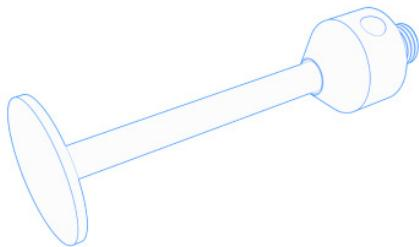
Disc styli are used, among other things, to measure rotationally symmetrical workpieces with undercuts or recesses and cylinders. However, a strong filtering of the surface roughness usually occurs. With the design of the spherical disk stylus, a higher accuracy is achieved compared to disk styli.
