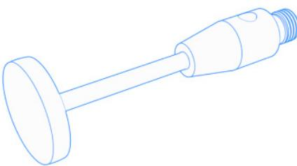
Disc styli are used, among other things, to measure rotationally symmetrical workpieces with undercuts or recesses and bores. However, a strong filtering of the surface roughness usually occurs. With the design of the spherical disk stylus, a higher accuracy is achieved compared to disk styli.
