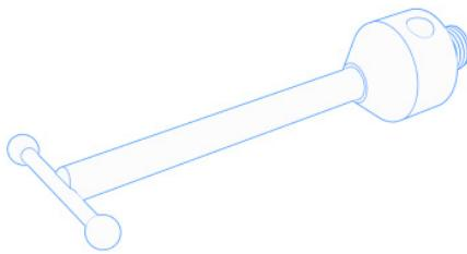
T-styli consist of two opposing measuring probe spheres mounted at 90° to the shaft. These styli are particularly suitable for measuring opposing holes and undercuts, such as grooves. In addition, T-styli can also be used for measuring points that are difficult to access (e.g. on the underside of the workpiece).
