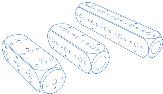
Multiple holders are milled stylus holders that are available in different designs. From beams to complex angular elements, almost any shape can be realized. Due to the high complexity of the requirements, the standard portfolio in the M5 range is limited to the most common shapes. Greater flexibility can be achieved by using M5 pro elements.
