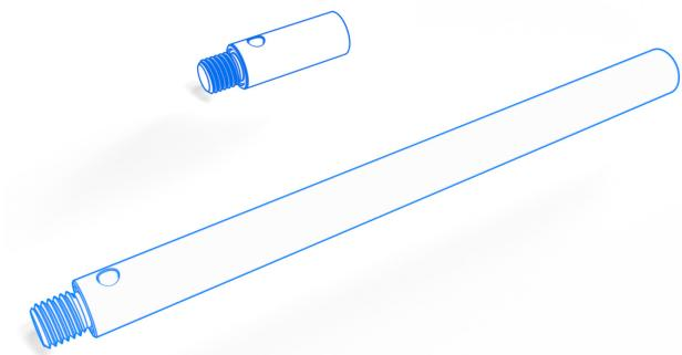
Standard M3 extensions have a smaller outer diameter of 4 mm compared to the 5 mm diameter used with the ZEISS M3 XXT system. The resulting loss of rigidity is compensated for by the use of a stable titanium rod. The weight of these extensions is lower than comparable extensions made of stainless steel, but still significantly higher than ZEISS M3 XXT systems
