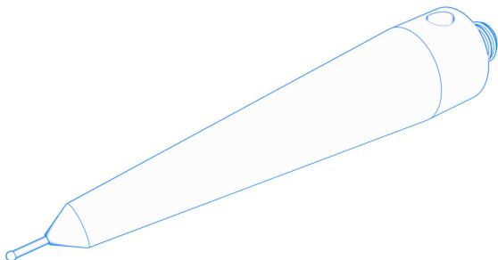
Cone shaft styli have an enlarged adapter that tapers only just before the stylus tip. This results in significantly better stiffness values for the entire stylus. Conversely, the usable length is reduced to the actual measuring length, since the conical contour subsequently provides a disturbing contour.
