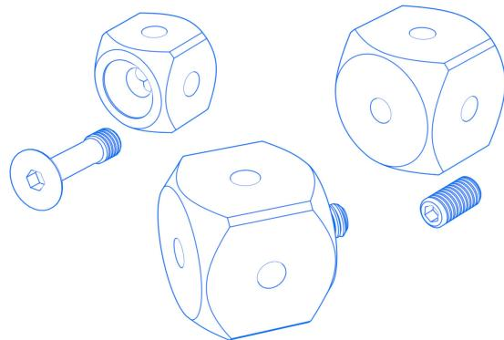
Cubes are the most common connection element in a stylus system.
