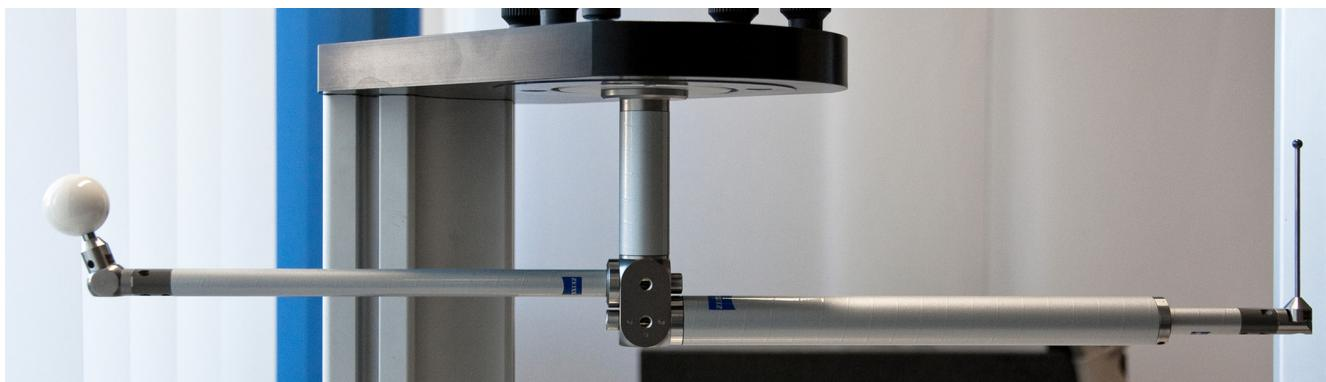
During the tactile measurement of a workpiece, many features may be difficult to access. For these cases a stylus extension can be used. While metal extensions are acceptable for touch trigger sensors, carbon fiber is a better choice for tactile scanning sensors.
