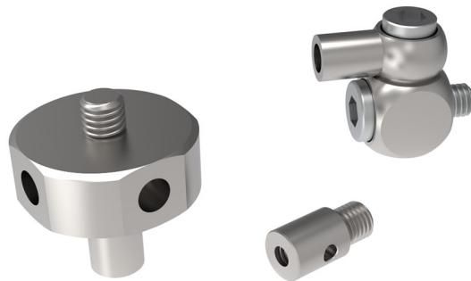
M3 REN connecting elements are used to create multiple or angled styli combinations and star styli with an M3 thread. The M3 REN system is based on 4 mm diameter base bodies and can only be combined with the M3 XXT system in exceptional cases using special adapters.
