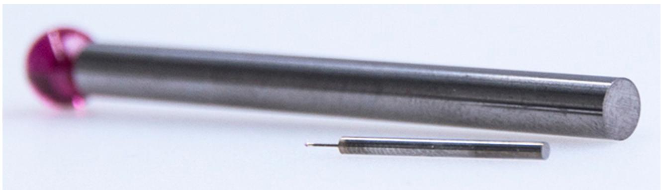
ZEISS threaded styli are used to measure even the smallest characteristics of parts. They are fastened in corresponding stylus holders. The stylus tip is made of either ruby or silicon nitride of the stylus shaft and consists of hard metal as standard. Styli without thread can be combined with the suitable connecting elements to form different configurations, e.g. L, T and star styli.
