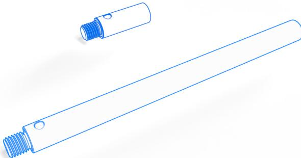
Standard M3 extensions have a smaller outer diameter of 4 mm compared to the 5 mm diameter used with the ZEISS M3 XXT system. The resulting loss of rigidity is compensated for by the use of a stable stainless steel rod. However the weight of the extensions is significantly higher compared to the carbon fiber used in the ZEISS M3 XXT system
