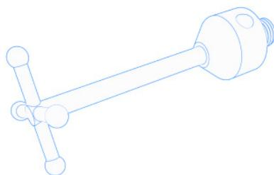
Star styli consist of spherical styli combined in a star shape and enable measurements in different coordinate directions. Whereas probing with spherical styli from the side surfaces is only possible to a limited extent, with the star stylus you can select the stylus for probing that is orthogonal to the probed surface.
