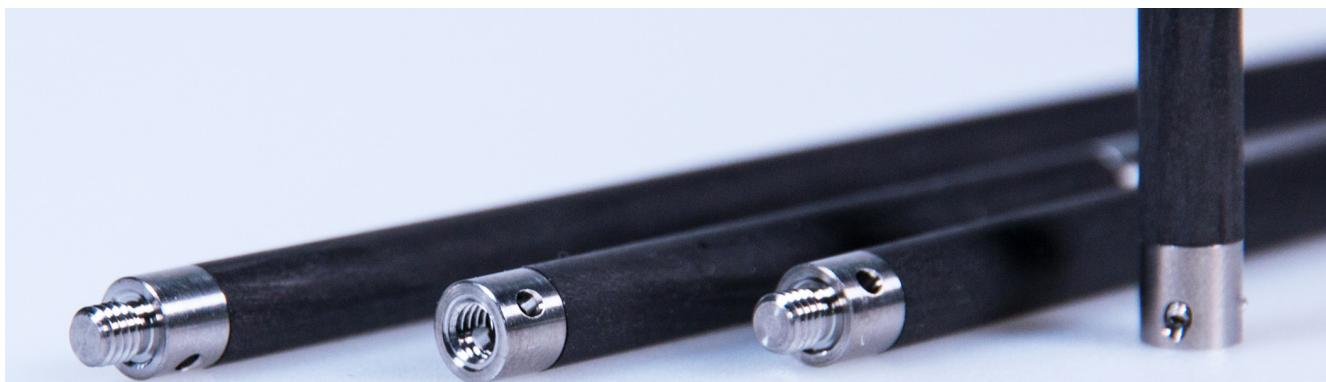
ZEISS REACH CFX®1 M3 XXT extensions have been specifically developed for the ZEISS VAST XXT measuring sensor. These extensions consist of carbon fiber tubes exclusively wound for ZEISS. At five millimeters, the diameter is larger than that of conventional M3 variants. This improves the contact surface and enables the extremely light, rigid construction. This supports the functionality of the measuring sensor - allows the highest possible accuracy.
