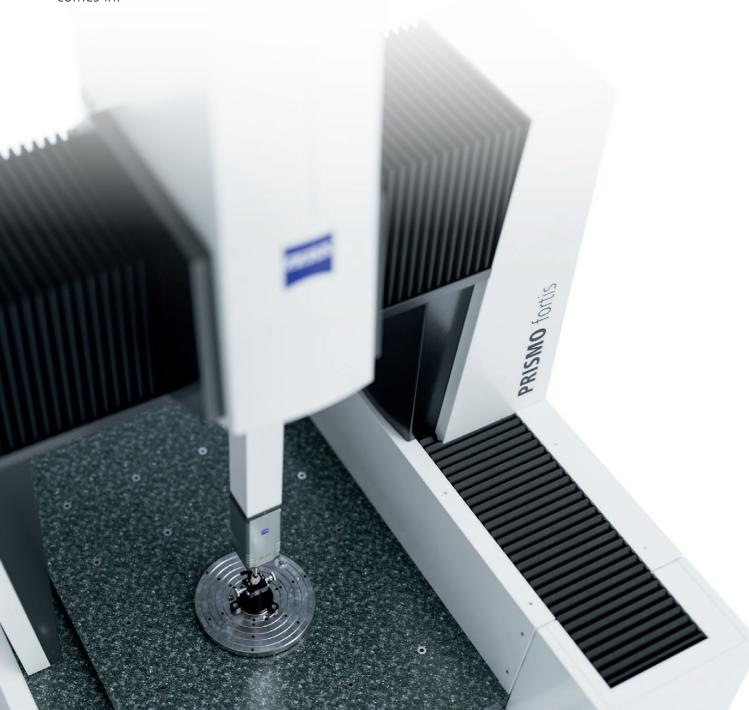
Available for ZEISS PRISMO 7/12/7 fortis, ZEISS CMM Acceleration Mode for Aerospace Applications comprises a pair of options known as ZEISS VAST Rotary Table Axis (ZVRA) and ZEISS VAST Rotary Table (ZVR) as well as a dedicated application support package if required. ZVRA ensures accuracy by providing swift definition of the axis of the rotary table, while ZVR promotes faster movement of the rotary table and thus faster measurement.
