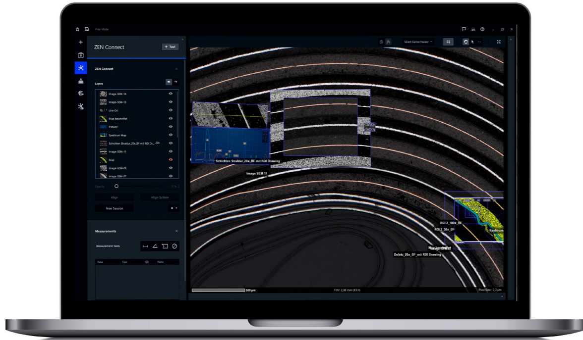
ZEISS ZEN Connect enables correlative image presentation from different microscope types (e.g. light and electron microscopes) in a connected map. This is highly beneficial for detailed investigation of large overview images, such as with battery cells.
