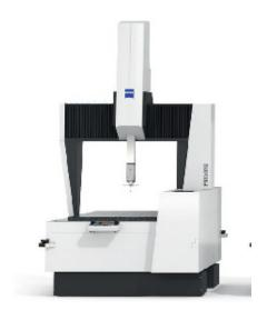
$0.5 + L/500 \mu m$ **Length measurement** 0.9 + L/350 µm error: MPE\_E0
