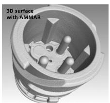
Artifacts caused by metal pins make proper evaluation or surface determination impossible.
