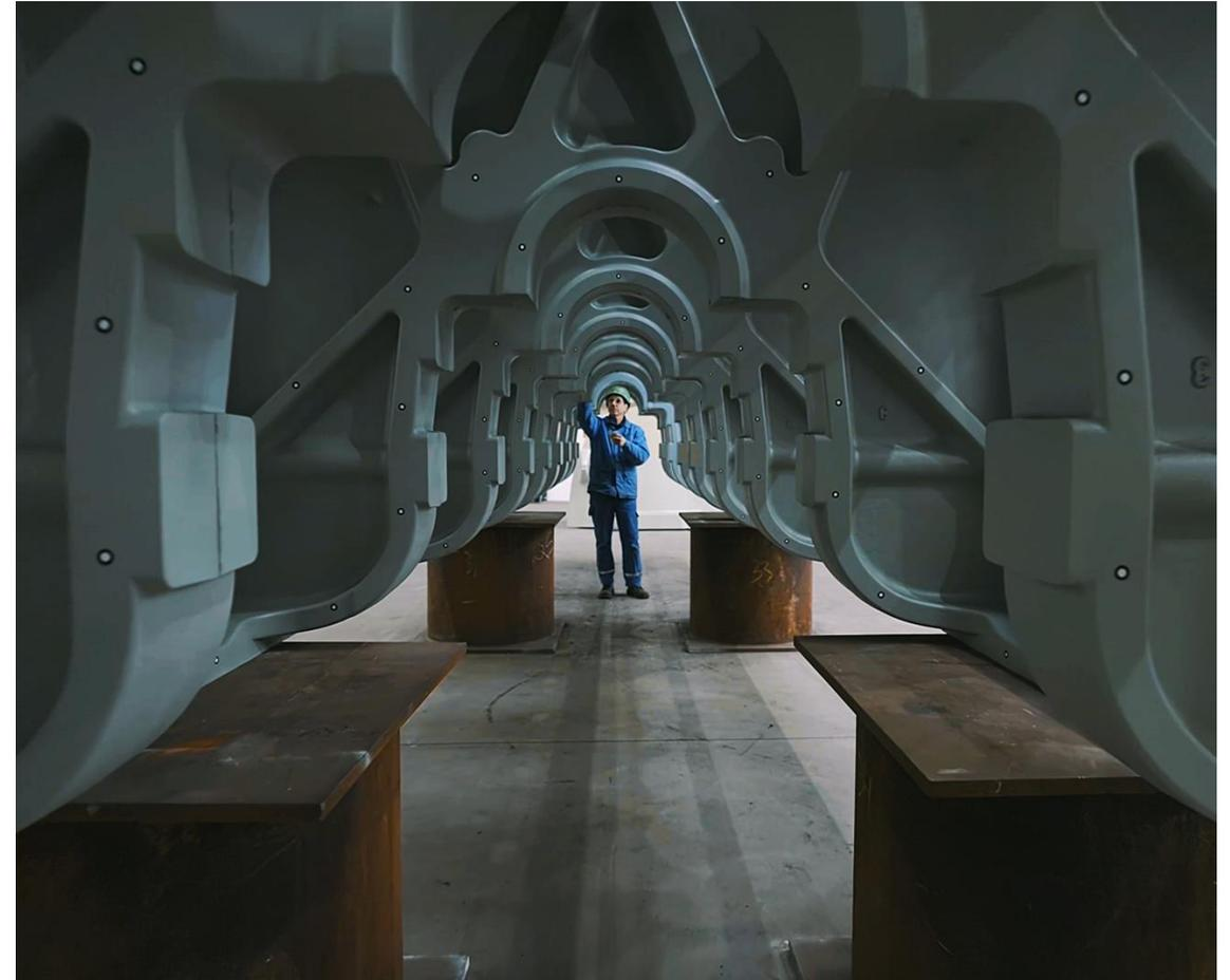
The German Siempelkamp Gießerei has installed the world's largest non-contact robot measuring cell together with ZEISS, to ensure precise quality of their very large castings.
