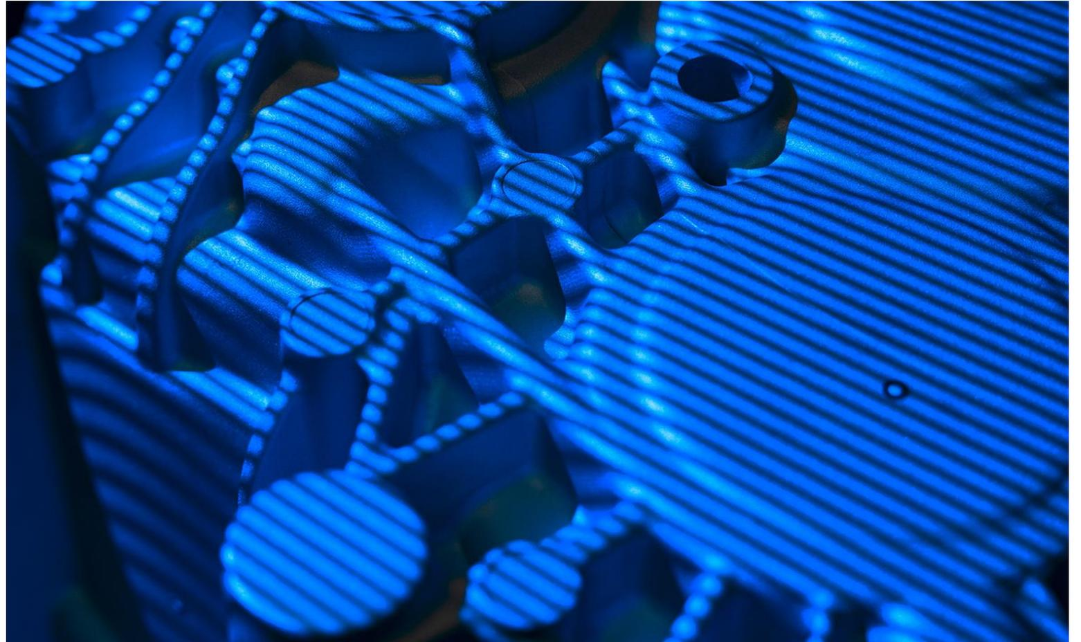
The principle of triangulation combined with the fringe projection technique enables the stereo camera system to capture precise 3D coordinates.
