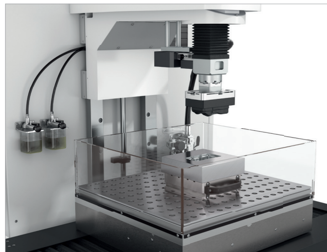
Measurement on the EDM machine yields a lower production volume, since long EDM machine setup times result.
