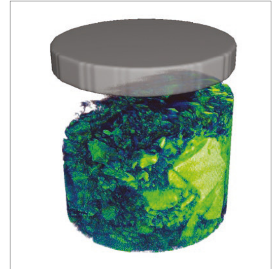
Elastomer at different stages of compression during an in situ load stage experiment (left: uncompressed, middle: compressed, right: after compression). Imaged with Xradia 810 Ultra (scale bar applicable on all three images).
