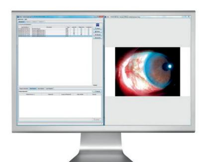
ZEISS FORUM LINK net converts data from non-DICOM instruments into a DICOM-compatible format.
