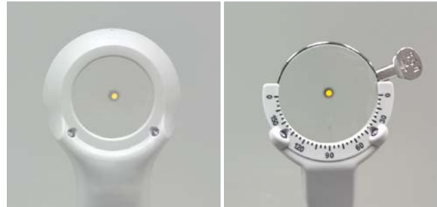
Image 2: The Liquid Trial Lens in comparison to the manual trial lens holder. The aperture of the Liquid Trial Lens on the front side is approximately 28mm and 34mm on the back side. The manual trial lens holder has an aperture at the front and the back of 34mm. In both lens systems, it is the back aperture that limits the field of view.
