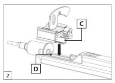
Ensure the plunger is fully retracted. Insert the loading chamber (C) containing the lens into the BLUEMIXS 180 injector (D).
