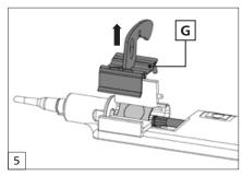
Remove vertically the safety cap (G). Visually verify the correct position of the lens.
