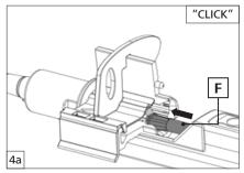
Gently push the plunger forward in the intermediate stop position towards the pin of the safety cap (F) until an audible "click" is heard. Pushing the plunger into the intermediate stop position is mandatory to ensure the lens remains in the intended position while removing the safety cap.
