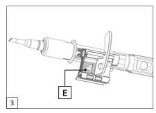
The triangle on the cap shall point towards the injector tip (E).
