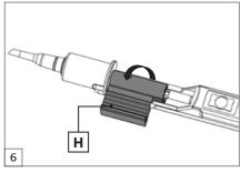
Close the loading chamber (H). The IOL is now ready for injection. Push the plunger forward. Ensure that the blue silicone cushion does not by-pass the pin at the back of the safety cap to avoid lens dislocation. If excessive resistance is felt while pushing the lens forward, check that the silicone cushion is completely separated from the lens. This ensures that the trailing haptic is properly positioned in front of the cushion.
