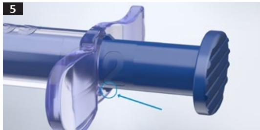
Slowly advance the lens until it has been released from the injector. If delivery is incomplete, apply additional pressure to the thumb flange to release the lens.
