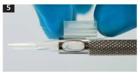
Guide the cartridge into the opening at the front end of the injector and push it to the very front position.
