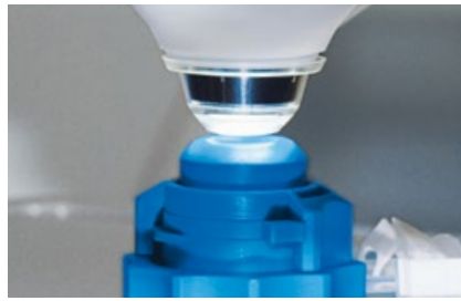
Specially designed curved contact glass (type KP) prevents unnecessary compression of the corneal tissue
