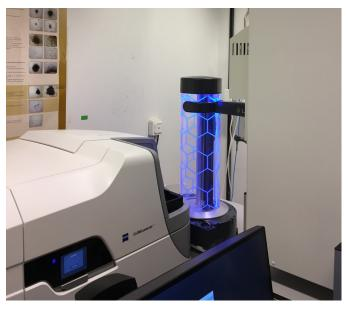
*Figure 1* Installation of S-LAB plate handler, Celldiscoverer 7 and incubator at a customer site
