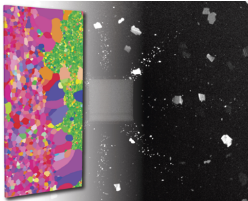
3D grain map of an ultra thin oriented electrical steel sample with dimension of (RD) 4 mm, (TD) 2 mm and (ND) 0.08 mm. Sample scanned using helical phyllotaxis HART scheme. Sample courtesy of Dr. Li Meng, China Iron and Steel Research Institute.
