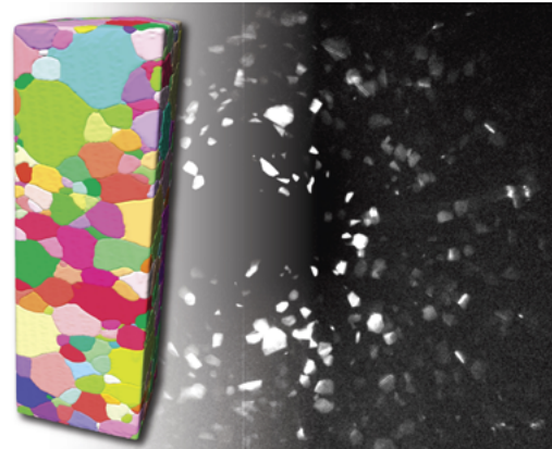
3D grain map of a \beta -Ti sample with dimension of (side length) 1.0 mm and (height) 3.2 mm. Sample scanned using helical phyllotaxis scheme.
