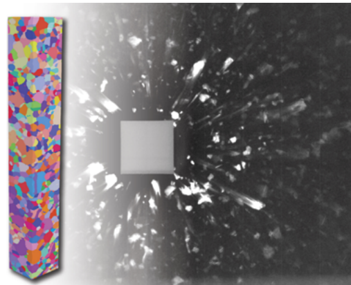
3D grain map of an austenitic stainless-steel sample with dimension of (side length) 0.66mm and (height) 4.4 mm. Sample scanned using helical phyllotaxis raster scheme. Sample courtesy of Prof. Grethe Wither, Technical University of Denmark.
