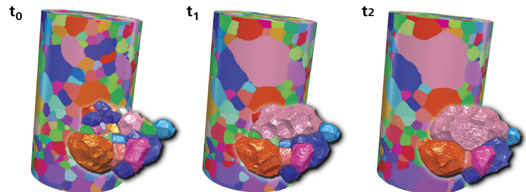
4D grain map of an Armco iron sample imaged at various annealing steps.
