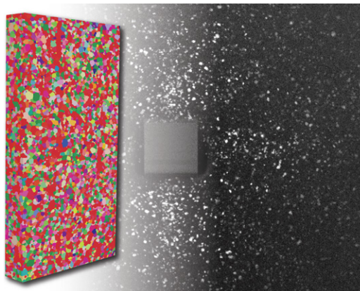
3D grain map of an AA5657 sample with dimension of (RD) 4 mm, (TD) 2 mm and (ND) 0.5 mm. Sample scanned using helical phyllotaxis HART scheme. Sample courtesy of Dr. Robert Sanders, Novelis, USA
