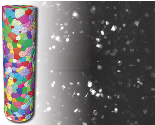
3D grain map of an Al-4wt.%Cu sample with dimension of (diameter) 1.1 mm and (height) 5.1 mm. Sample scanned using helical phyllotaxis scheme.
