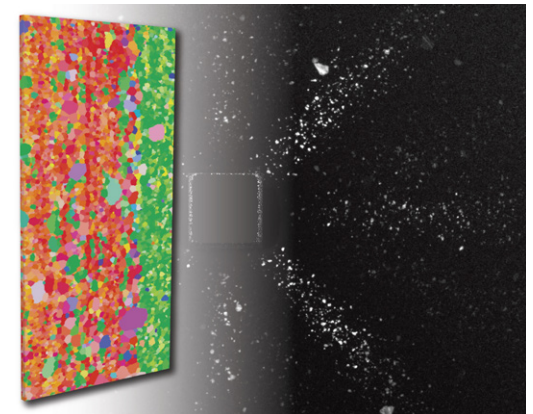
3D grain map of an ultra thin oriented electrical steel sample with dimension of (RD) 4 mm, (TD) 2 mm and (ND) 0.08 mm. Sample scanned using helical phyllotaxis HART. Sample courtesy of Dr. Li Meng, China Iron and Steel Research Institute, China
