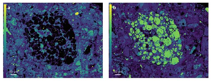
*Figure 2 a-b)* Close-up quantitative EDS maps (Fe and Mg) of an olivine aggregate chondrule seen within the sample in Figure 1. *Pure Fe-metal inclusions can be seen within the most pristine parts of the forsteritic olivine.*
