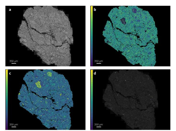
*Figure 1* a) SEM BSE image shows the complex, predominantly fine-grained sample of the Winchcombe meteorite; b-d) quantitative EDS maps of Fe, Mg and S (overlaid on BSE) allow instant visualization of difficult mineralogy even in complex samples. Even with no previous mineral library, all variations can be taken into account for further assessment, e.g. with automated mineralogy.
