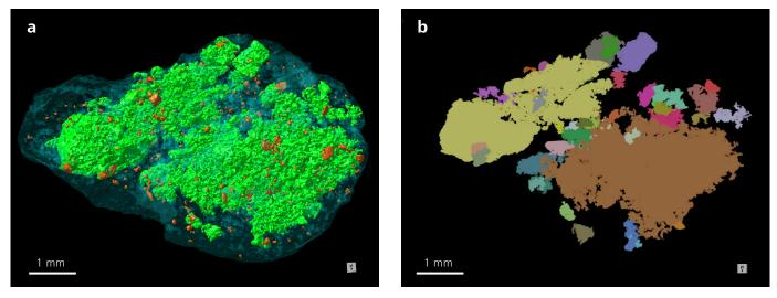
*Figure 3* a) Segmentation following deep learning-assisted reconstruction allowed clasts (green) and matrix (pale blue) to be separated. Sulfide and oxide minerals (orange-red) were also characterized using 3D automated mineralogy with ZEISS Mineralogic 3D. b) Size, distribution, and shape analysis of clasts give insights into collisional processes happening on the initial parental body from which the Winchcombe meteorite originated.
