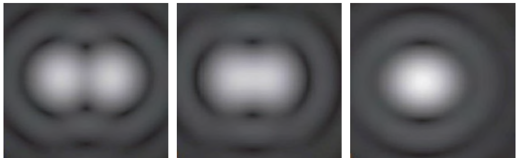
Figure 2 Spatial Resolution as a Function of Feature Separation. As the same pair of features becomes separated by spacing smaller than the resolution of a system, it becomes indistinguishable as a pair by the imaging system.
