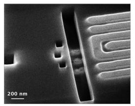
Rectangular hole milled through approximately 300 nm of dielectric to expose buried copper lines in a semiconductor chip. Fabrication: neon, imaging: helium.
