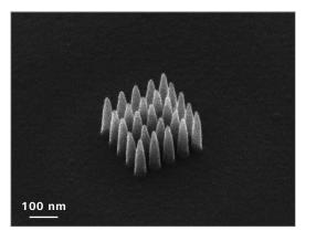
Array of platinum nano-pillars (pillars: 35 nm diameter, tight array pitch: 50 nm), example of the helium ion beam deposition capability. Fabrication and imaging: helium.
