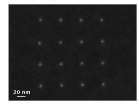
Scanning transmission electron micrograph of an array of 4 nm diameter nanopores drilled through a 30 nm silicon nitride membrane. Pores were drilled in about 1 second each. Fabrication: helium, imaging: electron. Courtesy of A. Hall, JSNN.
