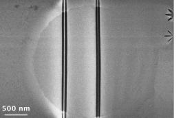
20 nm (left) and 10 nm (right) suspended nano-ribbons in graphene created by ion milling. Fabrication and imaging: helium. Courtesy of D. Pickard, National University of Singapore.
