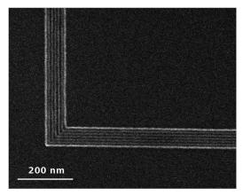
6 nm nested lines in HSQ fabricated by helium ion lithography. Courtesy of: HP Labs
