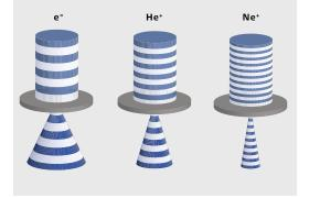
The helium and neon ions have a DeBroglie wavelength that is much smaller than an electron beam resulting in much less diffraction.
