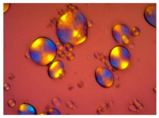
**Figure 2** Wheat starch (40×) with bimodal distribution. Small granules have a size between 2  $\mu$ m and 15  $\mu$ m, large granules between 25  $\mu$ m and 40  $\mu$ m. Courtesy of L. Prange, Crespel & Deiters GmbH, Germany
