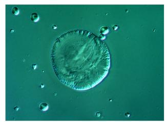
**Figure 9** Starch oxidized with sodium hypochlorite (40×). Courtesy of L. Prange, Crespel & Deiters GmbH, Germany
