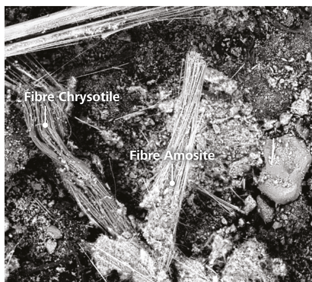
Amosite and Chrysotile detected
