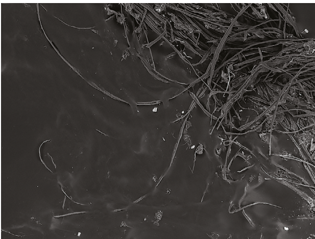
Asbestos paper (Chrysotile detected)
