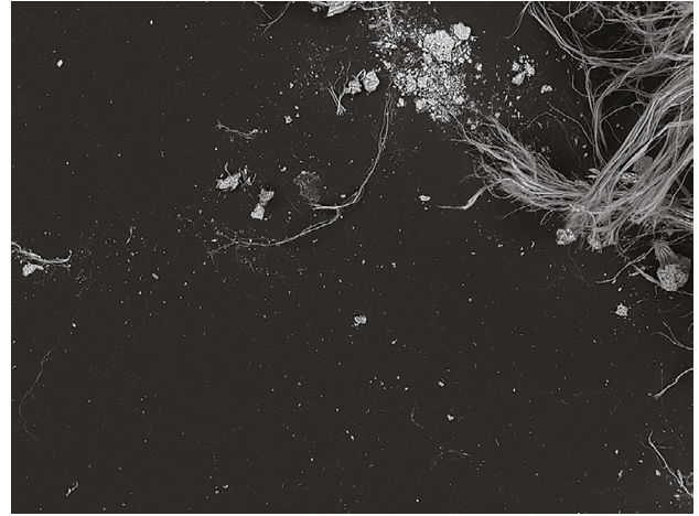
Asbestos cement (Chrysotile detected)
