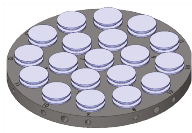
Figure 1 Carl Zeiss 19 stub multi holder carousel
