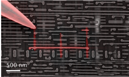
EBAC trace of logic nets in a sample showing underlying connectivity.
