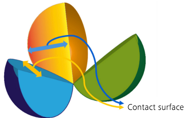
Figure 8 Particle split open to reveal the contact surfaces between minerals. It is the proportion of the surface to the total surface of the mineral in the sample that determines the level of association between the minerals.
