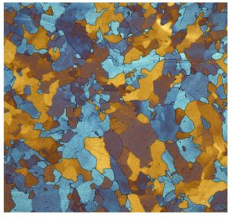
Pure iron in brightfield, reflected light, acquired with ZEISS Axio Observer, objective: EC Epiplan-APOCHROMAT 50× / 0.9
