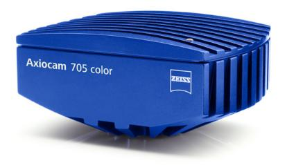
This flexible 5 megapixel scientific color camera strikes the perfect balance of speed and resolution. Delivering more than 60 frames per second at full 5 megapixel resolution, this camera captures even the most dynamic processes without compromising image resolution. Subsampling or sub-region readout accelerate your acquisition speed to hundreds of frames per second.
