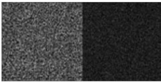
Dark Noise (Thermal Noise): origin by thermal electrons in the CCD cooling about 8 – 10° reduces dark rushing by factor two
