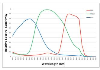
Spectral Sensitivity of ZEISS Educam 105 (incl. IR Filter)
