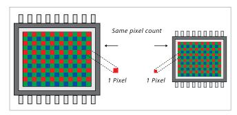
Even when the pixel count is the same, the image taken with the larger-sized pixels is less noisy because the CCD sensor is larger.
