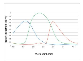
Relative spectral sensitivity ZEISS Axiocam 807 color.
