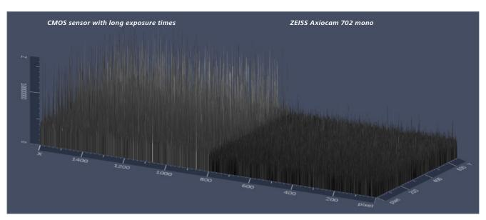
Left: Dark background, non uniformity from common CMOS sensor at 10s, Right: ZEISS Axiocam 702 mono with modern CMOS sensor at 10s with very dark background, low non uniformity
