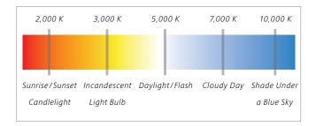
Color temperature is a temperature value (in Kelvin) of a light source and is used to describe the spectral characteristic of the corresponding spectral emission. It indicates the color impression of a light source: lower temperatures are more red, higher temperatures are more blue.
