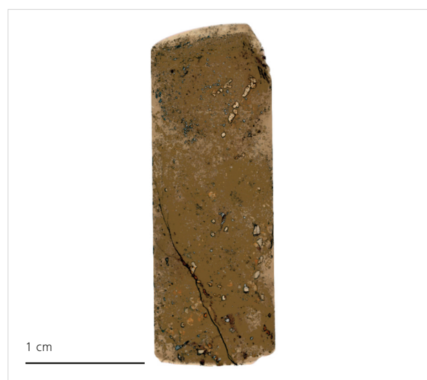
Figure 1 “Scout” view of the entire drill core (segmented to show the different mineral groups of silicates and sulphides).
