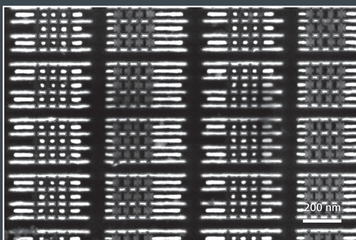
FinFET transistor. Top view, 22 nm technology, pure BSE imaging using EsB, at 3kV with high material contrast.
