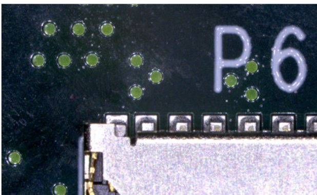
Figure 2a Features on a PCB revealing clear reflections from the segmented LED ring light (all switched on).
