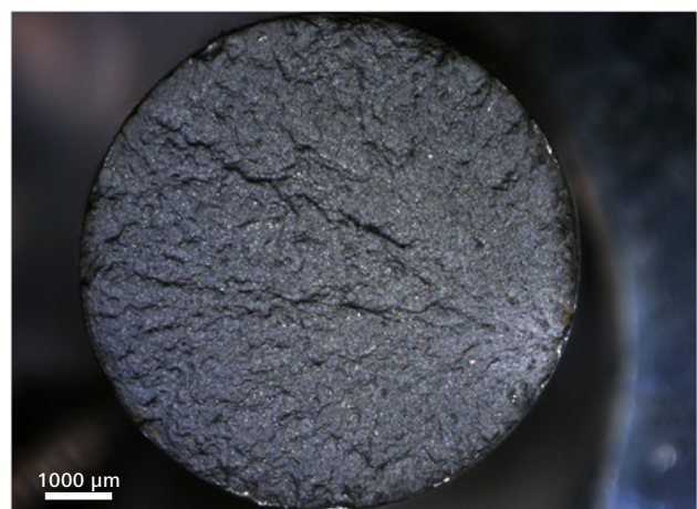
Figure 1c Overview image acquired with the digital light microscope of a metal rod fracture surface.
