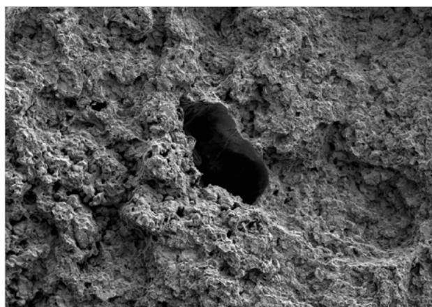
Figure 4a Secondary electron image of metal fracture, revealing sub-micrometer detail of the fracture surface morphology.
