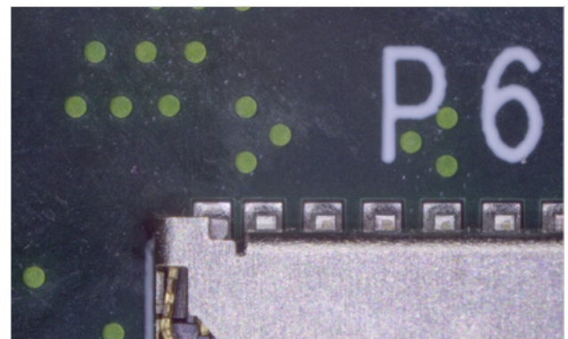
Figure 2b Same PCB now imaged with "glare removal" illumination settings that suppress the reflections visible in Fig. 2a.
