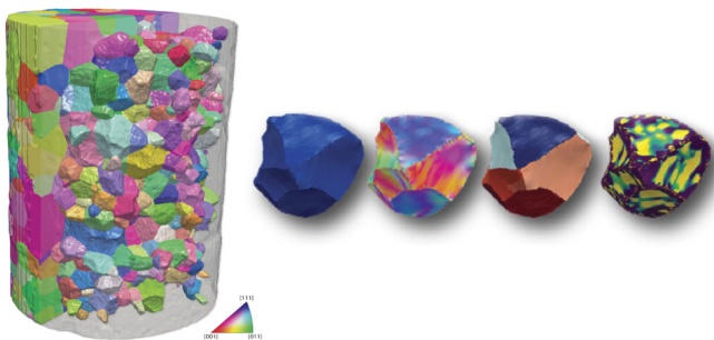
3D grain map of an Armco iron sample. Half the sample volume is removed to reveal inner grain (small clusters). Faces of a selected grain (left to right): by IPF color, grain boundary normal direction in crystal reference system, misorientation to neighboring grains, and grain boundary curvature.
